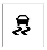
Pressing and holding the StabiliTrak® button located on the instrument panel for more than five seconds can turn off StabiliTrak® and part of the traction control system.
